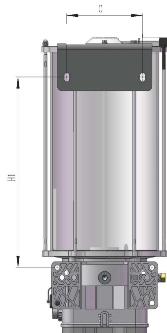
Dia. 19.3 Mounting dimensions for ALPB pump (Stirring paddle and spring piston type) on Top for Pump 15L ,20L and 30L.
